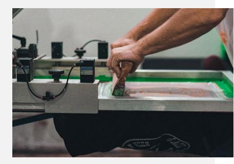
**Without pigment**, inks containing microspheres have a semi-opaque finish. For an **opaque white print** add up to 10% w/w titanium dioxide, and for a **coloured print** add up to 8% w/w non-ionic pigment dispersion.
