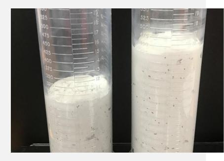
We showed **replacing** the **mineral filler** and/or **glass microspheres**, partially or fully, with **dry expanded microspheres** reduced the density of the putty.
