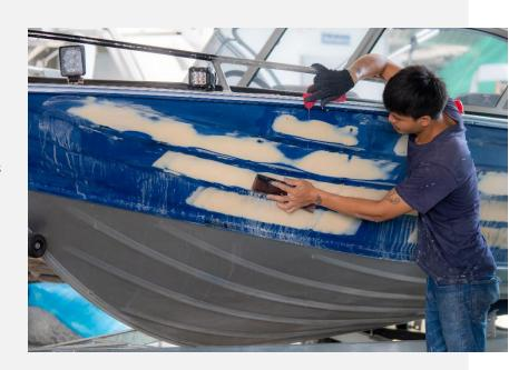
The quality of the finish is in the preparation, so after the repair surface has been carefully cleaned and sanded, coat the area just sanded with a thin coat of epoxy resin. This base coat acts as a key between the substrate and the fairing compound. The fairing compound is applied when the epoxy resin coat is tacky, but not fully cured.
