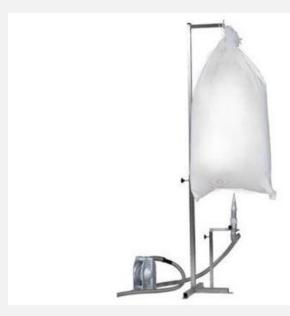
The handling system makes it easy to empty bags of dry expanded microspheres. It consists of a spear, diaphragm pump, metal hose (and couplings), air hose and stand.
